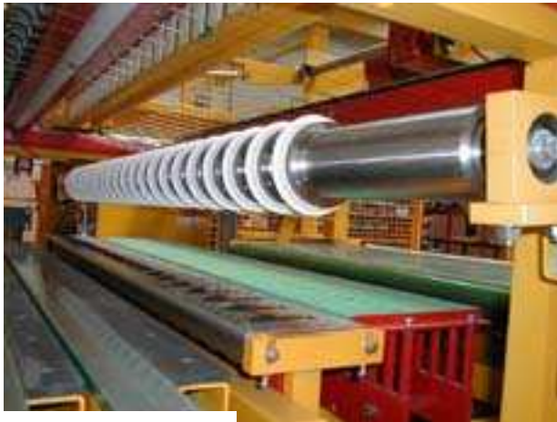
Multi-wire Cutter – Top Multi-cut Chamfering Device Cutting Out Bottom – Bottom left Multi-cut Slug Supply – Bottom right
